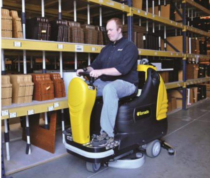
*A fully automatic floor scrubber is designed to apply cleaning solution to the floor, agitate or scrub it, wet-vacuum it, and then squeegee it dry, all automatically and all in one pass. Pictured here is the BD 26/27 Ride-On Automatic Scrubber.*
