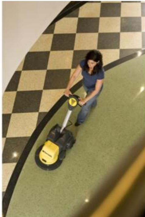
*A burnisher is a high-speed floor machine used to polish and clean floors. Pictured is the Battery Glazer 17 floor machine that operates on green batteries instead of a standard power cord.*
